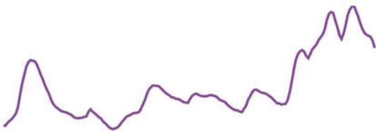
The Moodmetric smart ring detects the changes that can be followed online with the smart phone app. All the reactions cause an upward jump on the Scope, the bigger the reaction, the higher the curve goes. The physical response delay is 1.5 seconds, so the jump is visible 1.5 seconds after something makes a person react.
